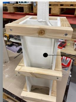
Structural steel **Column 02** prior to fire testing clad with 50X50mm timber strapping.
