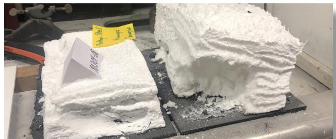
Photograph 1: Intumescent char expansion unrestricted during testing.
