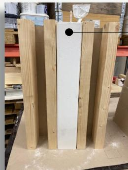
Structural steel **Column 02** prior to fire testing clad with 90x45mm timber framing and plasterboard hard against the steel face.
