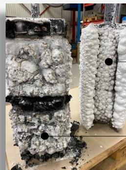
Structural steel **Column 01** (reference column) after fire testing.
