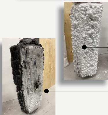
Structural steel **Column 01** (reference column) after fire testing.
